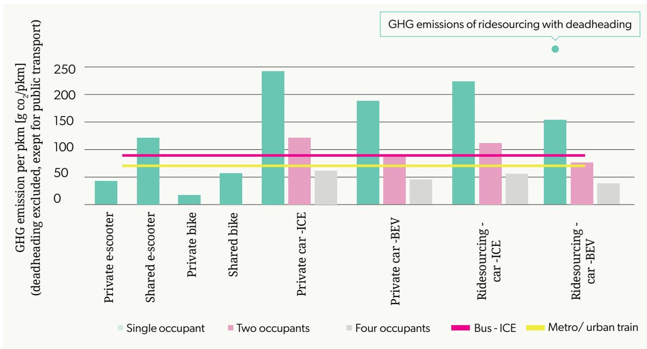
ICE is referring to internal combustion engine and BEV is an abbreviation of battery electric vehicle. If deadheading (cruising without passengers) is included (see top right side of the figure), ridesourcing becomes more CO<sub>2</sub>-intensive than using a private car.
