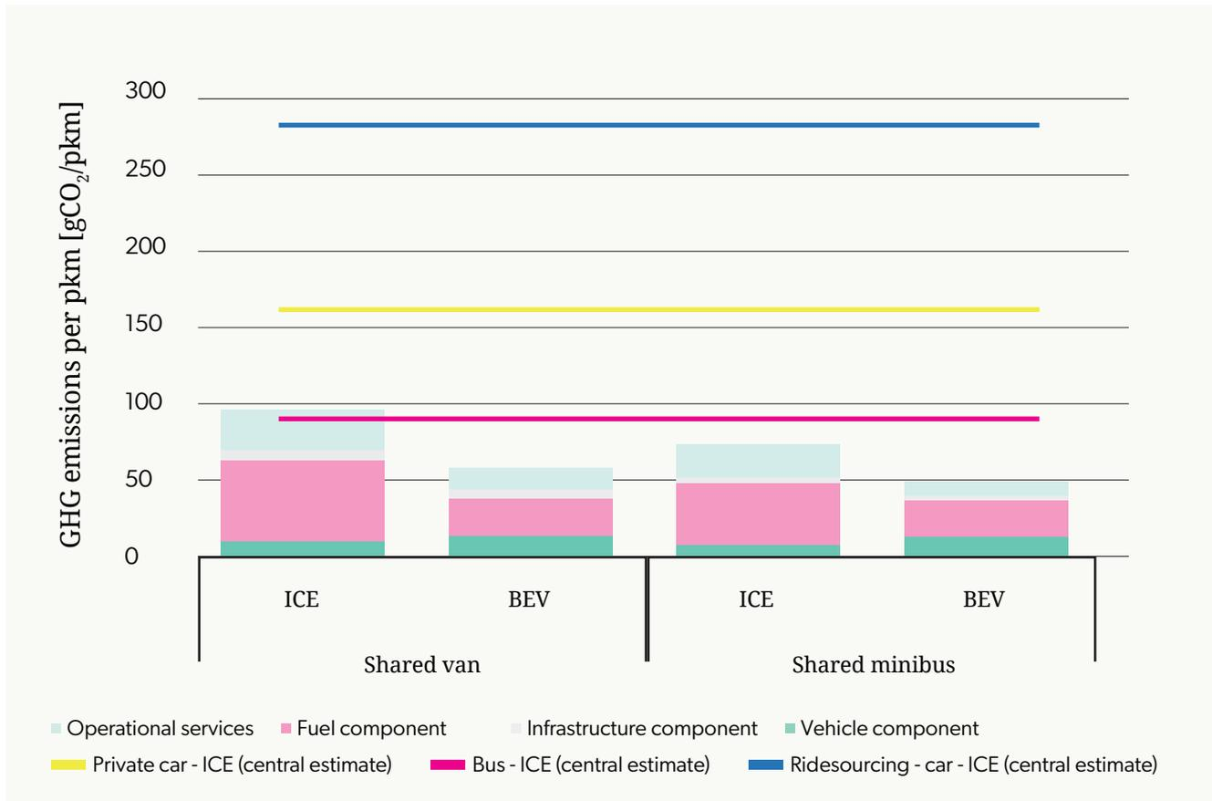
Vans are assumed to have eight seats, with a utilization rate of 70% as observed for New York City (4.5 seats occupied in average), and deadheading of 150%. Minibuses have a 20-seat capacity and average occupancy of 10 seats.
